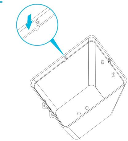
Attach the metal ring to the 4x hooks and press down to lock into place.
